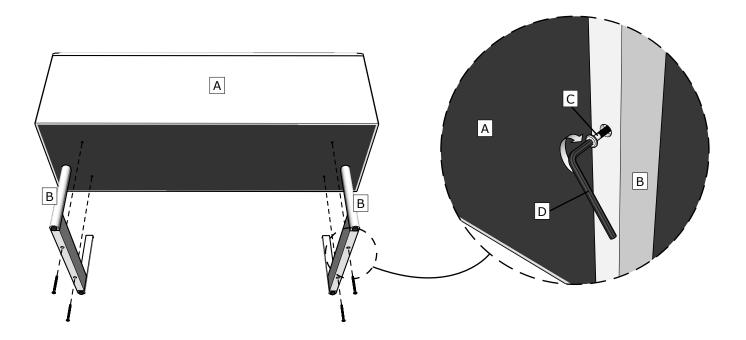
Attach  $\fbox{A}$  to  $\fbox{B}$  with  $\fbox{C}$  using a Hex Key Wrench  $\fbox{D}$  as shown.
