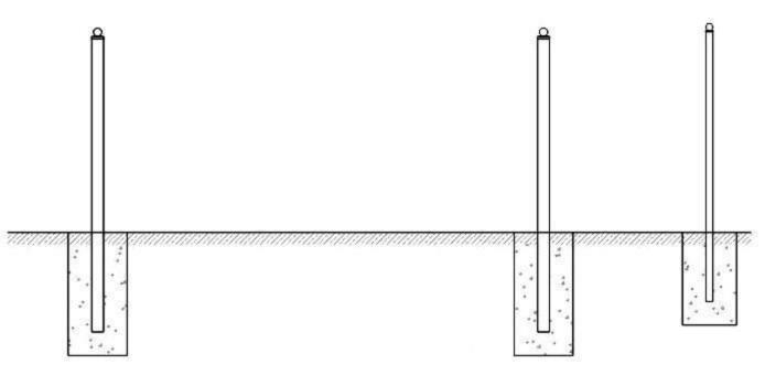
First step: Buried the posts, perpendicular to the ground.
