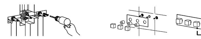
5. Install upper outlet pipe and top shower head. (wrap the PTFE tape on the thread)
