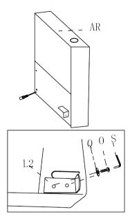
Step  $\,2\,$  Put the screws into the holes one by one. Please do not lock any one of the 3 screws before they are all aligned. After aligning them all and then tighten them with an electric screwdriver.
