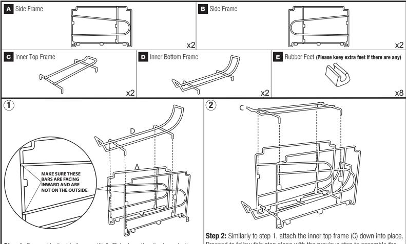
**Step 1:** Connect both side frames (A) & (B) by inserting the inner bottom frame (D) into place.
