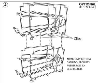
**Step 4:** If choosing to stack on top of one another, use the clips at the bottom top can rack to secure onto the bottom can rack. After making sure the can racks are secure, add any desired cans. Enjoy!
