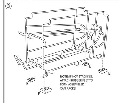
**Step 3:** Proceed to secure the rubber feet (E) accordingly to the bottom of the assembled can rack(s).
