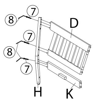
Insert dowels on Right Back Support Bar(K) and Right Backrest Panel(D) into mountings on Right Corner Leg(H) as shown above.
