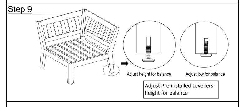
Inspect the Chair and make sure all parts are adequately connected.
