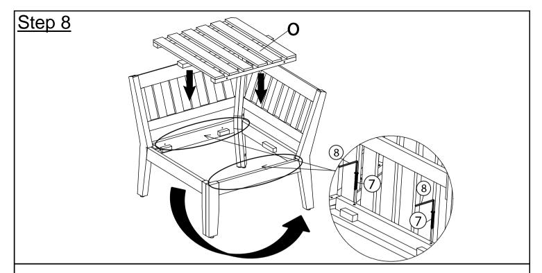
Insert the Seat Panel(O) into the Chair frame as shown in picture above. Attach Seat Panel(O) to Chair frame using Screws(7) with Allen Key(8). Note: Insert Screws(7) from inside to outside of Seat Panel(O). Do not fully tighten the Screws.
