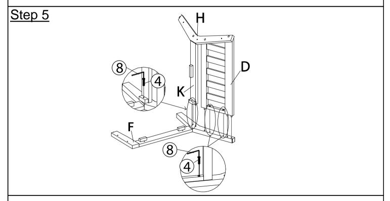
Insert dowels on Right Back Support Bar(K) and Right Backrest Panel(D) into mountings on Right Panel(F).
