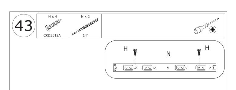
Fix rail(N) to board 3 with screw(H) at first.
