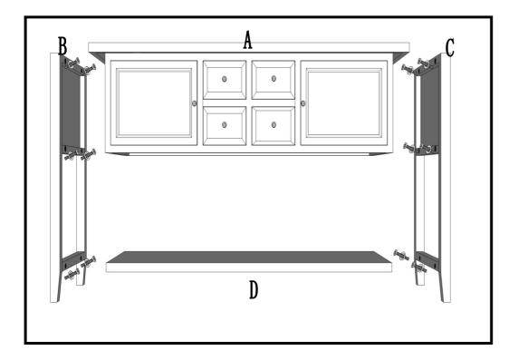
**Step 1**Attach the legs (B), (C) to the table top (A), use allen key to tighten the bolts(E). Then attach the shelf (D) to the legs, use allen key to tighten the bolts(E).
