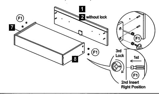
STEP 4 Use Screw (A2) to assemble the Single Plastic Cap (R2) to secure a bottom drawer panel. Assemble 5 sets of drawer in repeated at step
