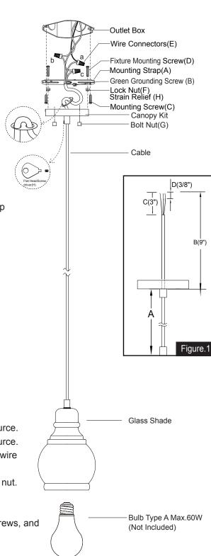
The following parts are available for re-order if damaged or missing.
