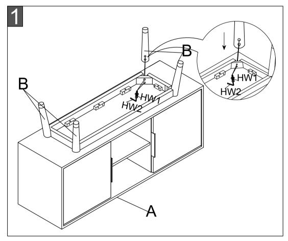
Step 1: Attach 4\*legs (B) in the corresponding position on the underneath of drawer (A) by using Allen key (HW2) to lock with 8\*Hex socket bolt (HW1). As picture.
