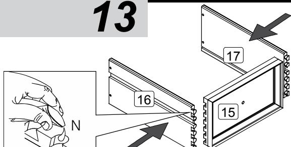
"Join drawer sides to drawer fronts with caution not to damage dovetail joints. Tap gently up and down the drawer side until fully inserted into drawer front."
