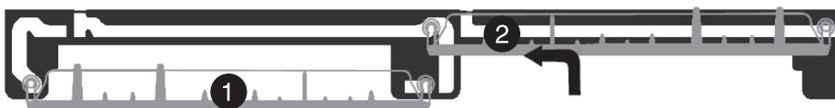
Left rack adjusted to lower position and right rack to upper position
