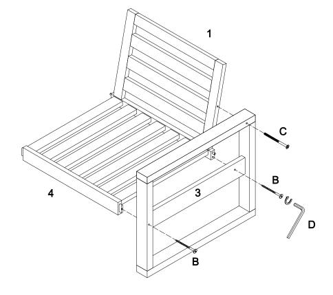
Use Wrench (D) to secure side frame (3) to seat frame (4) and back frame (1) with screw (B) and bolt (C).
