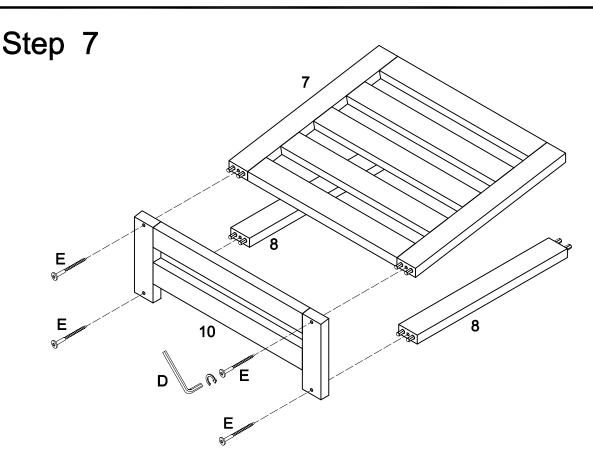
Insert top frame (7) and part (8) into side frame (10), then use wrench (D) to secure side frame (10) to top frame (7) and part (8) with screw (E).
