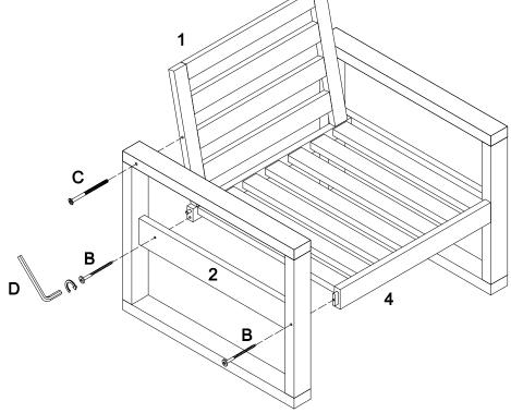
Use Wrench (D) to secure side frame (2) to seat frame (4) and back frame (1) with screw (B) and bolt (C).
