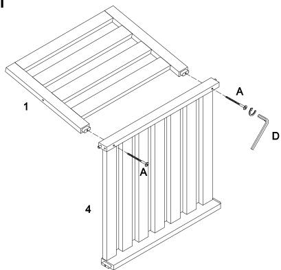
Use Wrench (D) to secure seat frame (4) to back frame (1) with screw (A).
