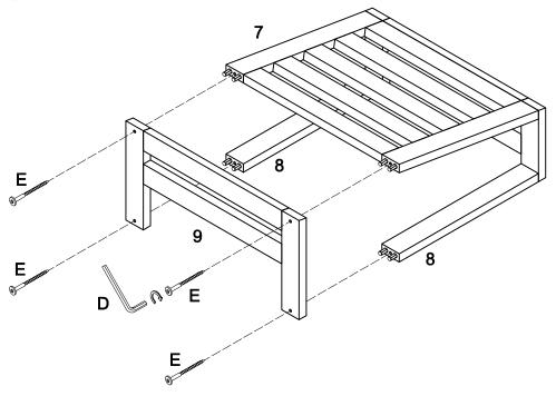
Insert top frame (7) and part (8) into side frame (9), then use wrench (D) to secure side frame (9) to top frame (7) and part (8) with screw (E).
