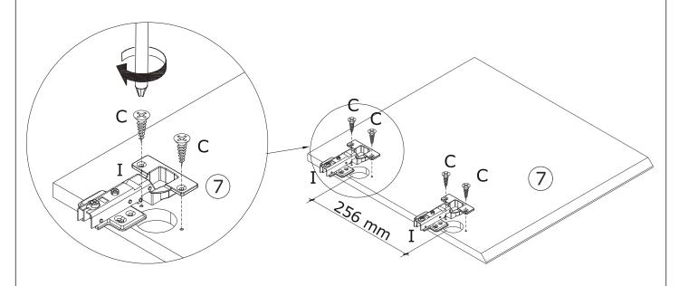
Fix hinge(J) to plate 8 using screw(C).
