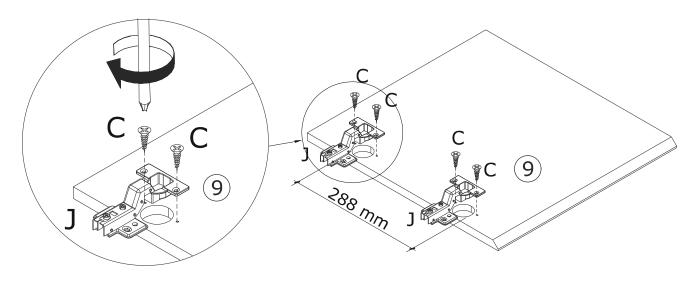
Fix hinge(I) to plate 10 using screw(C).
