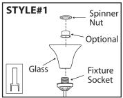
**STYLE#1** - Remove spinner nut from socket. Position glass on the fixture and secure with spinner nut. Install proper bulb type and wattage.
