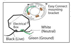
Attach easy connect mounting bracket to electrical box with electrical box screws (not included).
