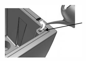
Remove fill port plug for direct access to the water reservoir.
