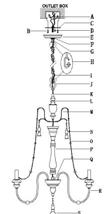
Step A1: Adjust arms (R) to the proper position, screw column (P) onto arms assembly (Q).
