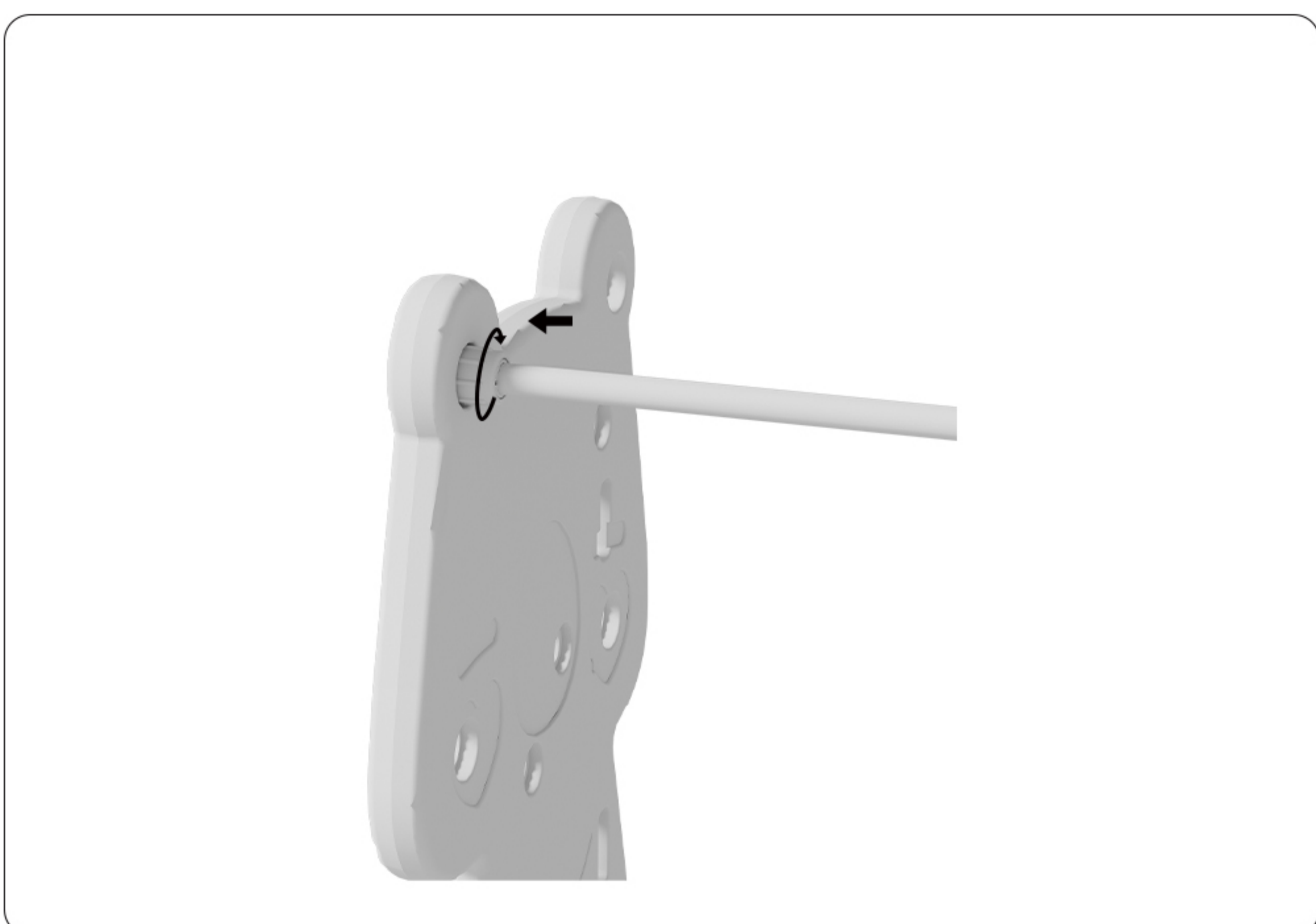
Step 5: Use installation tools to tighten accessory E (note that a nut needs to be used to clamp the nut on the other side). Other accessories should be assembled on the side panel in sequence according to steps 1, 2, and 3
