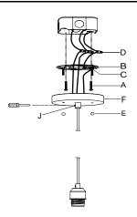
Step 3: Loosen the Allen screw (J) with a screwdriver, adjust it to the required length, attach the canopy of the lamp body (F) onto the mountirg plate (B), and secure it with round nut (E).
