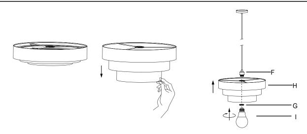
**Step 4:**Take out the lamp cover (H) and pull it down. Then install it on the lamp holder (F) and tighten it clockwise with the lamp holder ring (G). Insert the bulb (I) into the bulb holder
