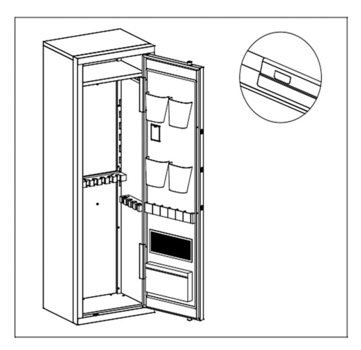
Install the shelf and snap the shelf into the grommet to complete the installation.
