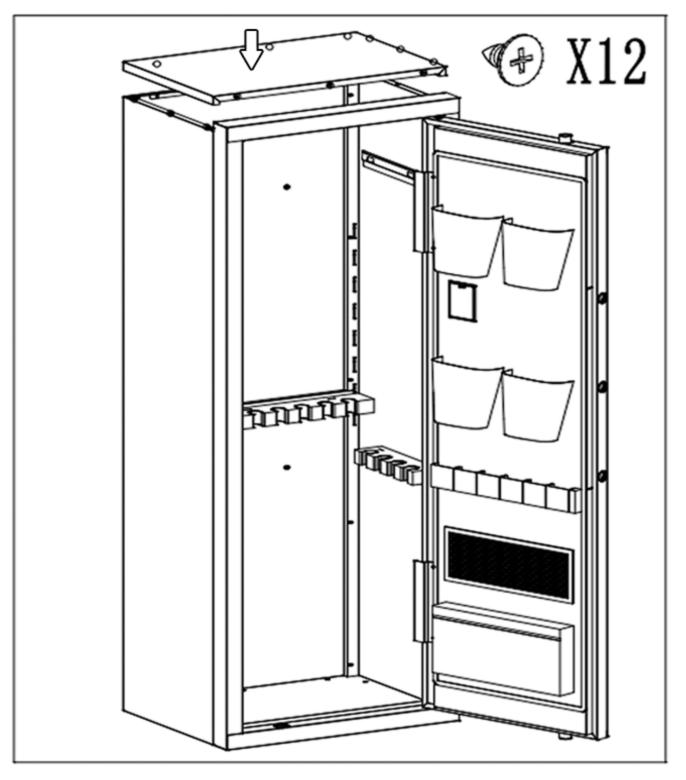
Install the top plate and connect it to the top with self-tapping screws.
