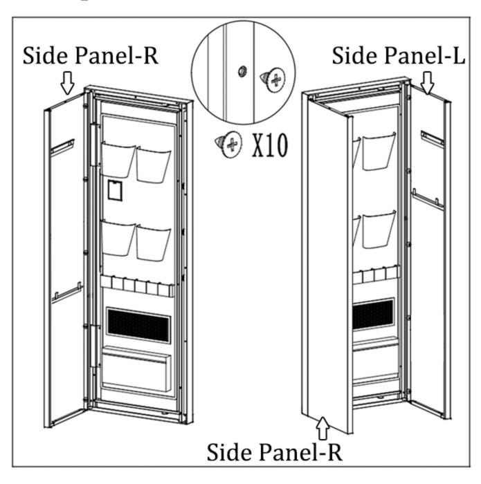
Connect the left and right side panels and door panels with self-tapping screws.
