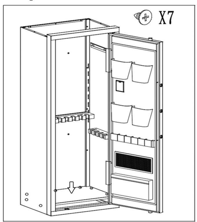
Install the bottom plate and connect it to the bottom with self-tapping screws.
