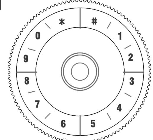
2. Enter any new 3-12 digits code, press the "#" button to confirm. The buzzer will sound once and the blue indicator light will be off. Password is set successfully.
