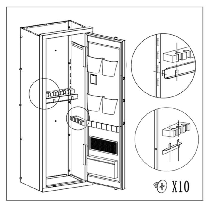
Connect the left and right side panels and back panel with self-tapping screws (open the door panel), and install an adjustable gun mount.
