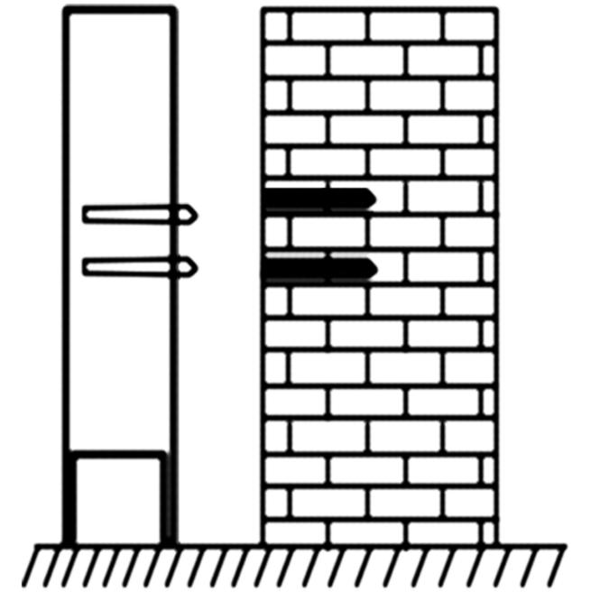
Expansion screws can be threaded through pre-drilled holes in the safe to secure it anywhere.
