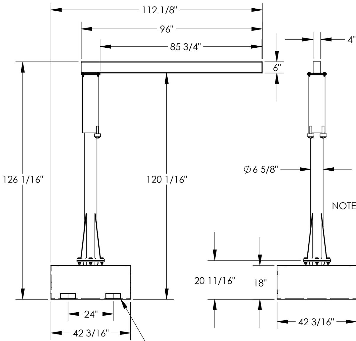
NOTE: UNIT IS FILLED WITH GRAVEL OR LIMESTONE AGGREGATE CONCRETE.
