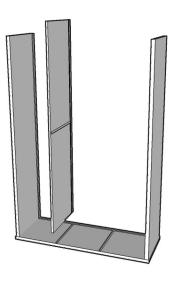
Step 4:Insert center shelf into remaining mortise of side piece, making sure notch faces back grooves of asembled pieces. Insert hex screws into each of (2) pre-driled holes in side piece and tighten down halfway.
