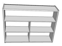
**Step 9:** Tighten down all scres until snug. DO NOT OVER TIGHTEN. DO NOT DRILL. rotate unit until it rests on **bottom** piece and edges of **side** piece. Assembly of first unit is now compete.
