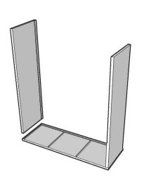
**Step 2:**Insert edge of **top** piece into mortise of **side** piece, making sure to align back grooves on all pieces. Insert hex screws in each of (2) predrilled holes in **side** piece and tighten down halfway.
