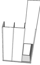
**Step 6:** Insert sides of back piece into back grooves of bottom piece and top shelf. Slide into place until edge of large back piece rests in back groove of side piece.
