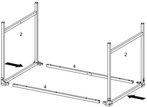
Insert the Side Frame (2) to the Support Bar (4).
