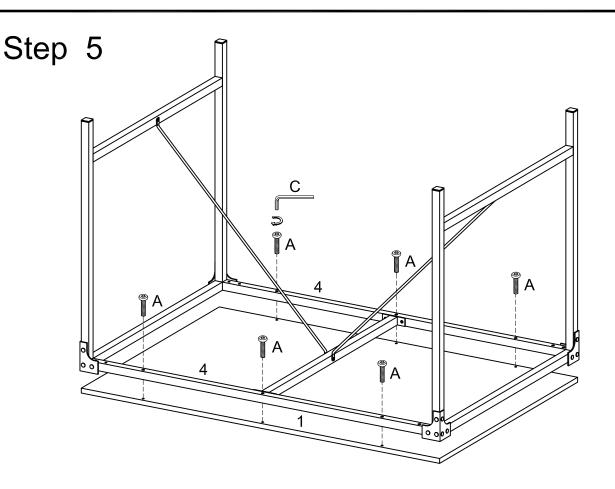
Use Wrench (C), Bolt (A) to secure the Support Bar (4) to the Top Panel (1).
