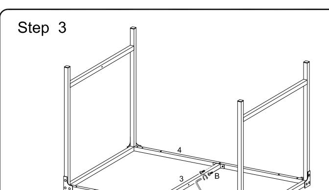
Use Wrench (C), Bolt (B) to secure the Cross Bar (3) to the Support Bar (4).
