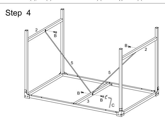
Use Wrench (C), Bolt (B) to secure the Wire Support (5) to the Side Frame (2) and Cross Bar (3).
