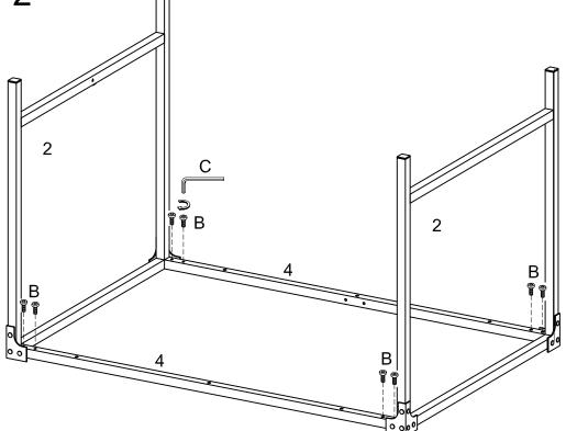
Use Wrench (C), Bolt (B) to secure the side frame (2) to the Support Bar (4).
