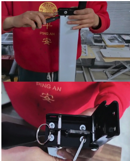
Step 1: Put the switch, handle and flip on the column and fix it with screw number 2
