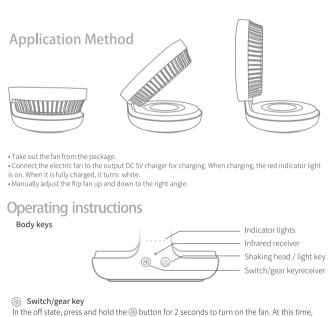
the fan will turn on the first gear speed, touch the (a) turn on gain to turn on the second gear speed, three times to turn on the third gear speed, four times to turn on the fourth gear speed, and five times to turn off the fan. Its corresponding indicator will light up and cycle Press and hold the
