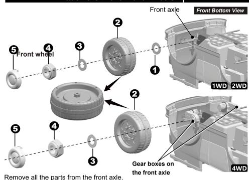
1. **1WD 2WD** type: Slide a **Ø10 washer** onto the front axle.
