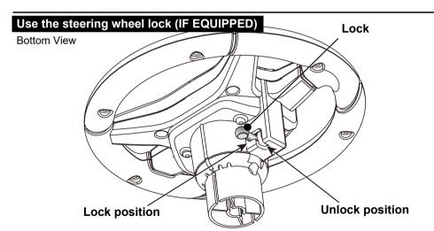
When the lock in the *lock position*, the steering wheel can control the direction of the vehicle.
