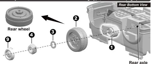
Remove all the parts from the rear axle.
