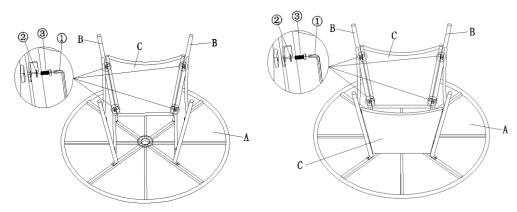
Align the holes in the Table Legs Support Panels (C) with the holes on the Table Leg(B). Affix the panels to the legs by using Washer (2) & Bolt (3) with Allen Key (1). Repeat the same steps to affix the other Table Legs Support Panels.
