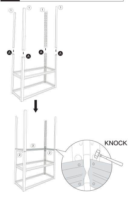
Step 8 Finish assembling the rest of cross bars as previous steps then install the plastic fastener for better robustness.
