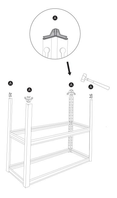
Step 7 Connect 4 vertical bars ( 1 ) to the finished frame by 4 connectors ( A ) , then connect the cross bars ( 2 & 3 ) as shown below.
