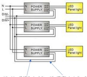
Connect the blue (0-10V) wire & the white (GND)wire to the dimmer
