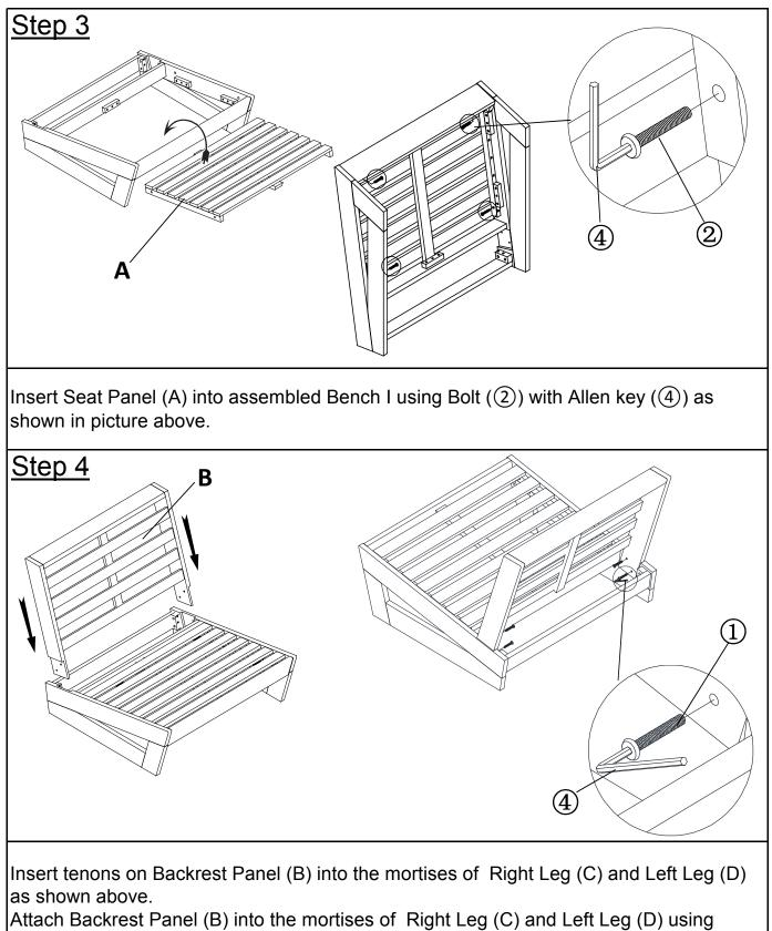
Bolt((1)) with Allen Key((4)) as shown in picture above.
