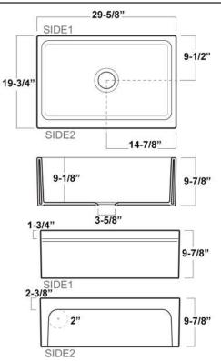
Dimensions of fixture are nominal and may vary within the range of tolerances established by ANSI Standard A112.19.2. Dimensions and specifications subject to change without notice.
