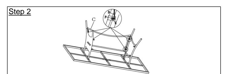
Attach Leg Support Panel(C) between Leg Panels(B) using Bolt(E) and Washer(F) with Allen Key(D) as shown in the picture above.
