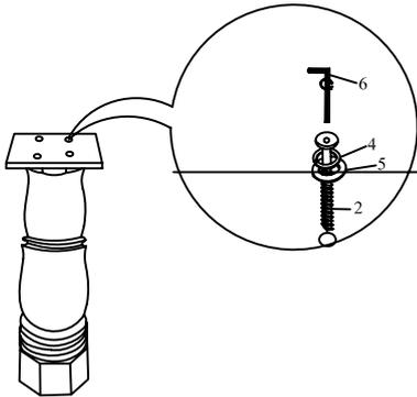
STEP 2: Put Assembled with Mounting Plate on the Bar , tighten with Flate(5), Lock washer (4) and Bolts(1) with Allen Key(6)
