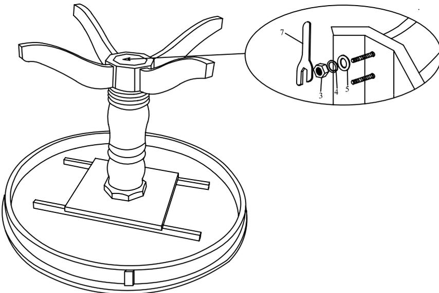
STEP 3: Attach the Leg (D) to the Pedestal (B), tighten all with Flat Washer (5), Lock Washer(4) and Hex Nut (3) with Wrench(7)
