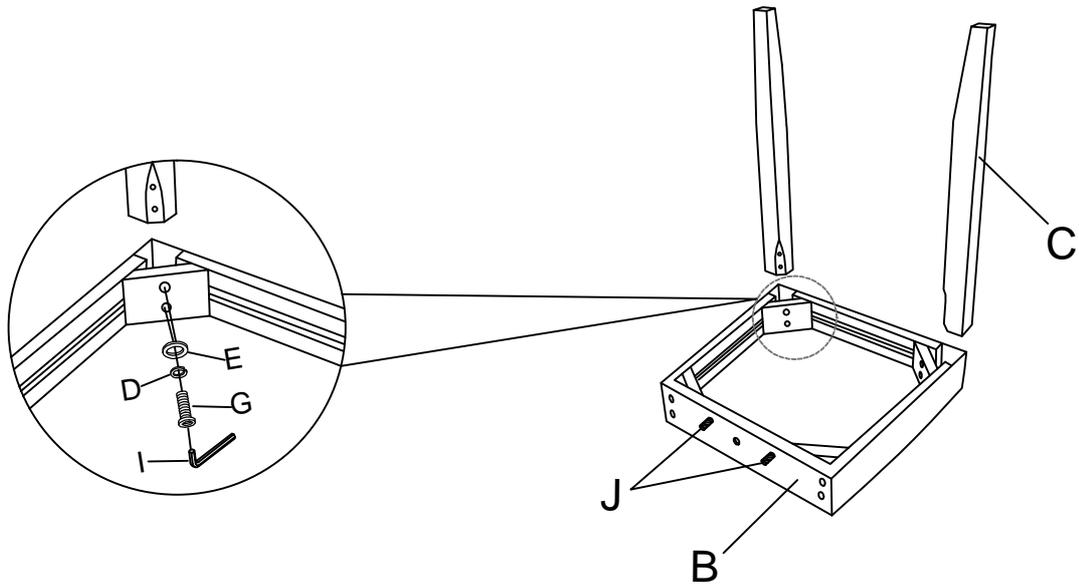
**2** Attach the Chair back(A) to Seat(B) with Wood plug(J), then lock them using Lock washer(D), Flat washer(E), Bolt(F) and Bolt(H) by Allen key(I).
