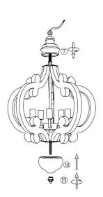
3.Let the wire go through the top cover ⑦, rotate to fix the cover ⑦ to the fixture, close the bottom cover ⑥ to the fixture with end cap ⑥.
