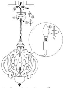
5.Install the bracket to the ceiling junction box with screw (3).
