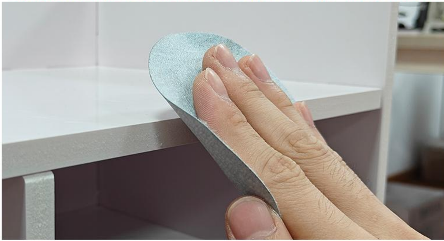
9.IF THERE ARE SHARP AREAS ON THE EDGE OF THE PLATE, THEY CAN BE POLISHED FLAT
