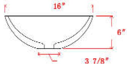
Dimensions of fixture are nominal and may vary within the range of tolerances established by ASME Standard A112.19.2. Dimensions and specifications subject to change without notice.
