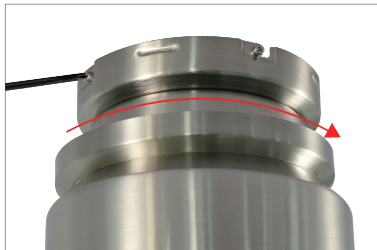
Step 5 Hang the motor on the mounting plate and rotate it until fixed.And then tighten the 4 screws.
