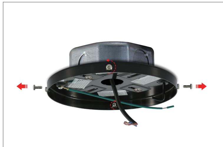
Step 3 Unscrew 2 opposite screws and loosen the other 2 opposite screws.
