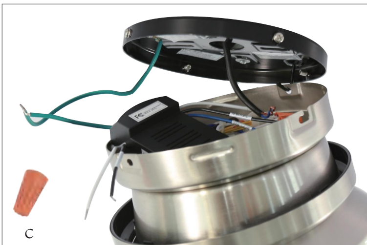
Step 4 Hang the motor on the mounting plate with the J-hook. Connect the home wires to the receiver. Black for Live Wire, White for neutral Wire,Green for Ground wire.
