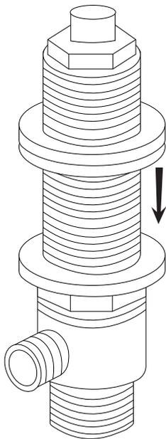
7. From under the countertop, insert the valve stem into the right-side faucet hole. From above the countertop, slide one of two decorative escutcheons onto the stem. Then, attach one of the two bell flanges to the stem by hand tightening until secure.
