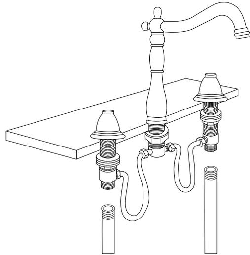
12. To complete the installation, install the faucet handles using a Philip's screwdriver.
