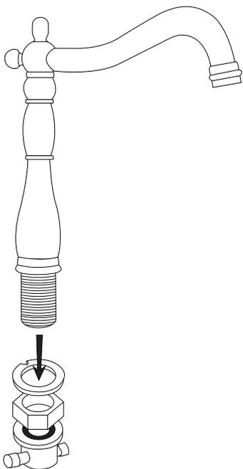
3. Set the spout into the center faucet hole. Position the decorative escutcheon so that the hole for the drain's lift rod is in the back.
