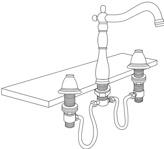
11. Attach the main water lines to the proper inlet on the bottom of each valve stem. Use an adjustable wrench to tighten, but be careful not to overtighten. Apply thread sealant or plumber's tape to each threaded connection. Ensure that you are connecting the hot and cold lines appropriately.
