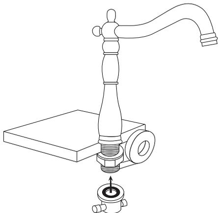
6. The faucet's valve stems are labeled by colored plastic washers - blue for 'cold' and red for 'hot.' On the 'cold' valve stem, loosen the lock nut to its furthest point at the bottom of the stem.
