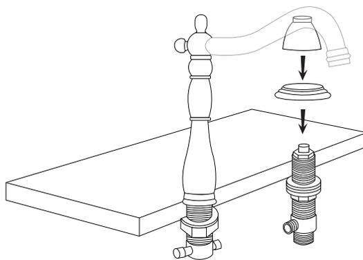
8. From beneath the sink, position the stem so that the outlet on the side of the stem is pointing inward, towards the T-connector. While holding in place, hand tighten the lock nut. Finish tightening using a basin wrench.
