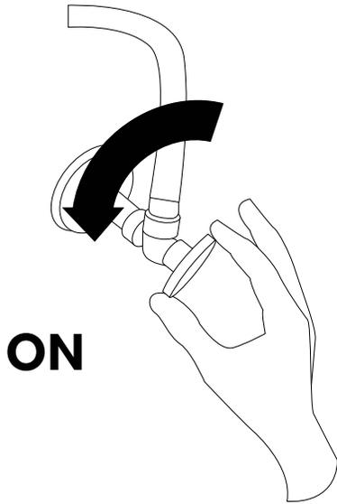
14. Remove the aerator from the spout and turn the faucet on for approximately 60 seconds to allow any dust or loose sediment to exit the water lines. Check for any leaks. Test both hot and cold water to ensure they are running properly. Once testing is complete, reattach the aerator.
