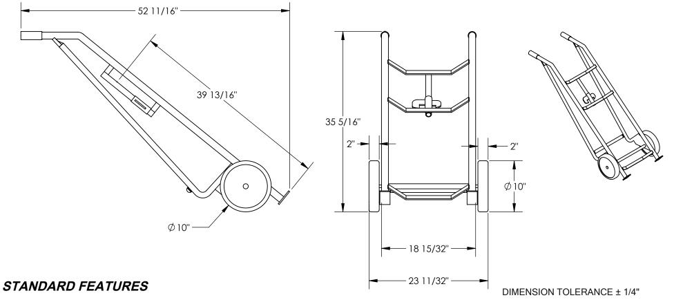
MODEL NUMBER IS DBT-RED OVERALL WIDTH IS 23 11/32" USABLE WIDTH IS 18 15/32" OVERALL LENGTH IS 52 11/16" USABLE LENGTH IS 39 13/16" OVERALL HEIGHT IS 35 5/16" MAX CAPACITY IS 800 LB 10" X 2" POLYURETHANE WHEELS
