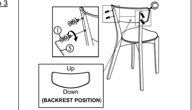
Align the Backrest(C) to Leg(A) and Leg(B) as shown above. Attach Backrest(C) to Leg(A) and Leg(B) using JCBC Bolts(1) with Allen Key(5). **Do not fully tighten the Bolts.**
