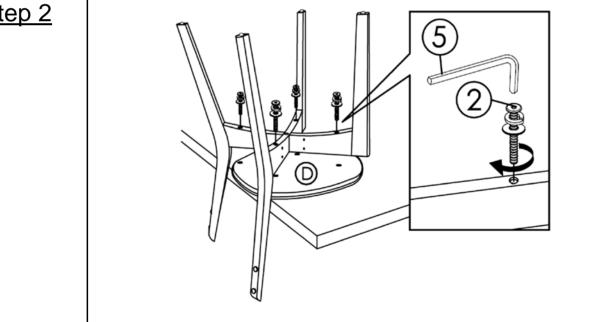
Place Seat Cushion(D) facedown on the edge of a table top as shown. Align Leg(A) and Leg(B) to Seat Cushion(D) as shown above.
