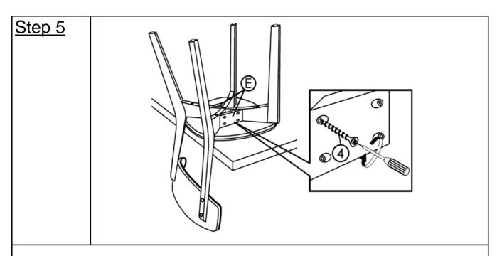
Place the Corner Block(E) at the side joint of Leg(A) and Leg(B) as shown. Attach Corner Block(E) to Leg(A) and Leg(B) using Screws(4) with Screwdriver(6). **Do not fully tighten the Screws.**
