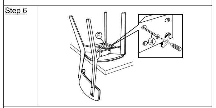
Place the Corner Block(F) at the front joint of Leg(A) and Leg(B) as shown. Attach Corner Block(F) to Leg(A) and Leg(B) using Screws(4) with Screwdriver(6). **Do not fully tighten the Screws.**
