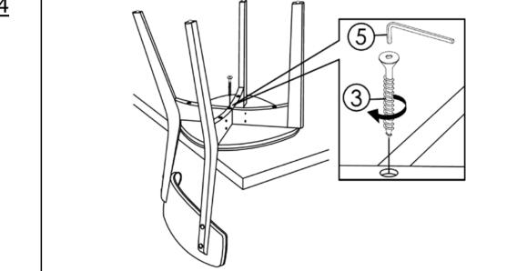
Attach Leg(A) to Leg(B) using JCBC Screw(③) with Allen Key(⑤) as shown. **Do not fully tighten the Screw.**
