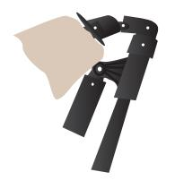
Hold the 2 clips together and fasten the canopy piece to the upright arm.
