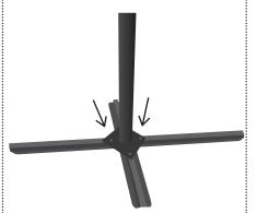
Using a 9/16 wrench and the bolts included, bolt the main umbrella support post to the base.
