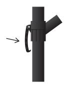
After placing the umbrella in the desired position, slide the black cap down and lock the safety handle.
