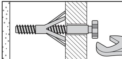
For use when fitting or supporting heavy loads such as shelving, wall cabinets and coat racks.
