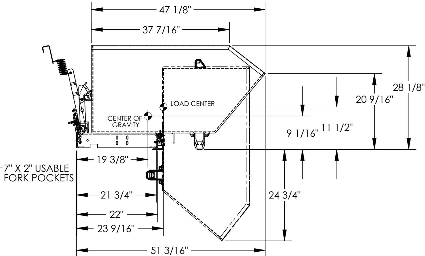
NEVER EXCEED LOAD CENTER RATING PER FORK TRUCK MANUFACTURER'S GUIDELINES. DO NOT USE THIS FORK TRUCK ATTACHMENT IF LOAD WILL EXCEED FORK TRUCK MANUFACTURER'S LOAD CENTER RATING.
