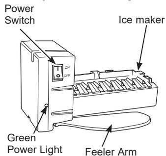
The ice maker will produce seven cubes per cycle approximately 100–130 cubes in a 24-hour period, depending on freezer compartment temperature, room temperature, number of door openings and other use conditions.
