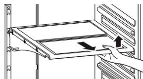
Quick Space Shelf (on some models) can retract to half its size for storage of tall items on the shelf below. Pull shelf out and up, slide shelf back until it stops to create half-shelf. Pull up and forward, then down to return to full shelf.
