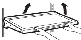
Lift up on the front and then up on the back to remove shelf.
