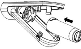
2. Line up the ports on the filter with the ports on the filter cartridge holder, and gently insert the filter.
