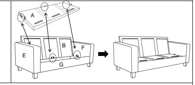
With assistance from your adult partner, hold up the Seat Base(A) on the top of the assembled parts, put the front side of Seat Base(A) over on the rail of Front Seat Board(G) as picture.
