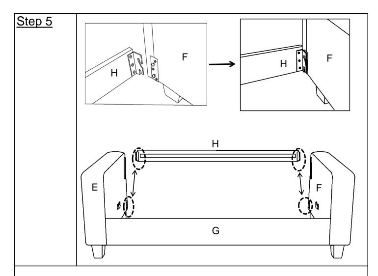
As to the Step 4, assemble the Hind Seat Board(H) at the behind of Left Arm(E) and Right Arm(F) as picture, don't need to tight with Allen Key.
