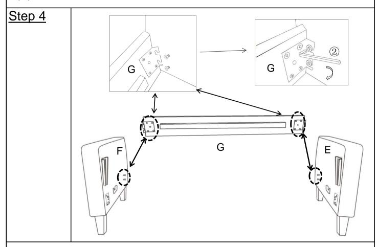
With assistance from your adult partner, postion the Left Arm (E) and Right Arm (F) as picture, hold up the Front Seat Board(G) and stand front the both Arms, assemble the Front Seat Board(G) by putting the metal hook on the two raised screws on the front side of both arms and push down make sure to the right position, then by tighten with Allen Key(②). do it one by one and make sure into position.
