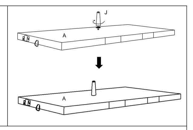
Install the Middle Leg with 1 Plastic Gaskets(J) at the bottom of the Seat Base(A). Insert threaded stem into the mounting position at the bottom of the Seat Base(A), Tighten by turning the Leg clockwise.
