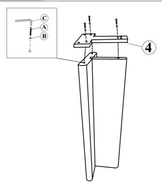
Don't tighten the bolts until all 3 bolts are slightly secured.
