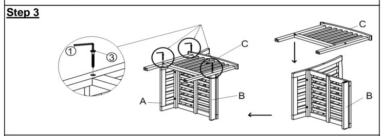
Attach Left Leg Panel (C) to Backrest Panel (A) and Seat Panel (B) using 3 Screws (3) + Allen Key (1).
