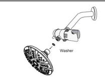
(5) Ensure the fixed showerhead is tightened to the diverter.
