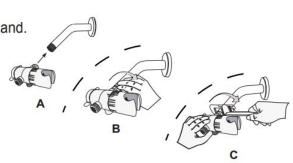
4 Ensure a washer is in the ball joint of the fixed showerhead.
