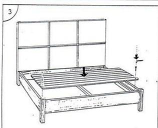
Put wooden mattrass support over the center wooden support, then lock using bolt M8x40 at each corner using allen key.
