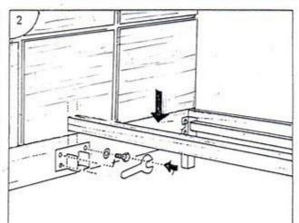
Install central plate to the Headboard and Footboard, then lock using bolt M8x20 turn it until tight using matching key, then pujt center wooden support over it.
