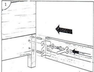
Insert all dowels to both end of Bedside then install this bedside to the Head-board & Footboard, lock using bolt M8x20 turn until tight using matching key.
